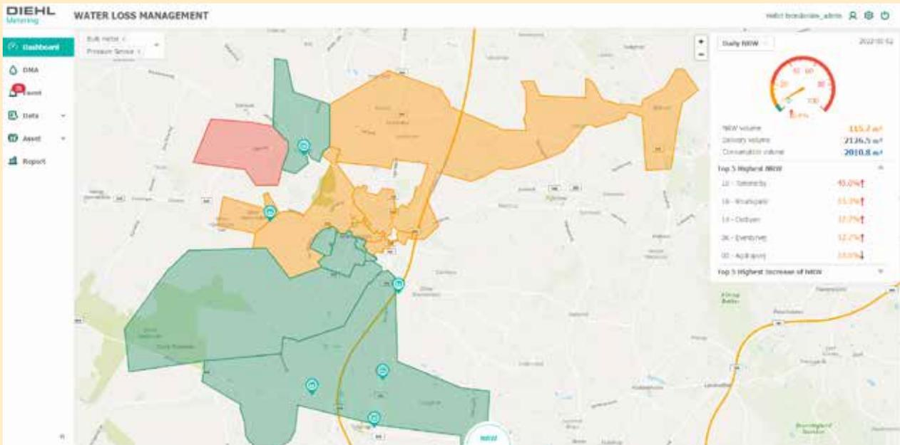
The green areas in the figure indicate that the water loss in the respective sections is less than 5 %. It is below 7.5 % in the yellow ones, and if the colour changes to red, the water loss exceeds 7.5 %.
